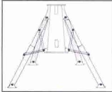
**Special Stabilizers** designed to reduce truck frame stress.
